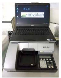
The kit is delivered as a microplate of 96 small cells. each enabling one analysis. The liquor to be tested is added to the cell, which changes colour. specific reader A linked to a laptop computer analyses the colour change, by 450 nm absorbance, and derives the phosphate concentration. The kit
