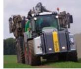
BioCover [www.biocover.dk](http://www.biocover.dk) Photo: slurry tanker equipped with SyreN
