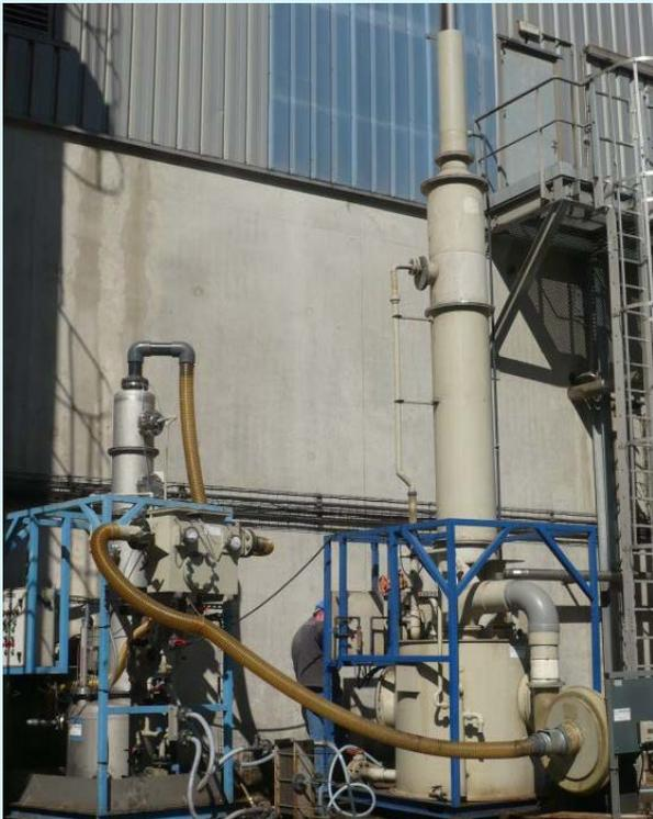
Stripper scrubber pilot at Waterleau New Energy plant in Ieper
