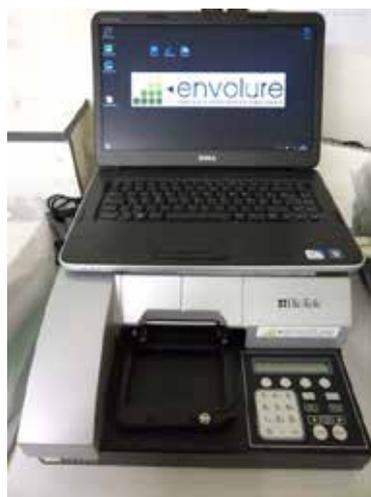
The kit is delivered as a microplate of 96 small cells, each enabling one analysis. The liquor to be tested is added to the cell, which changes colour. **A specific reader linked to a laptop computer analyses the colour change**, by 450 nm absorbance, and derives the phosphate concentration. The kit
