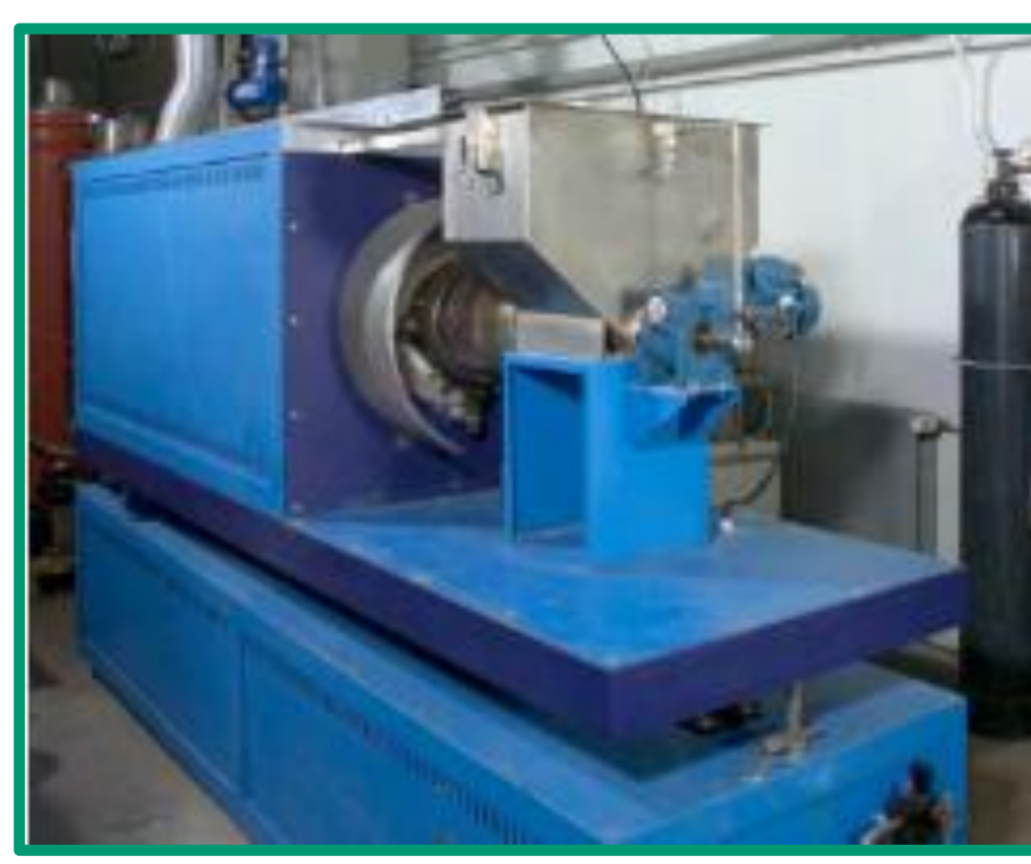
Fig. 2: Rotary furnace for TPT with HCl and Na 2 SO 4 , BAM Berlin.
