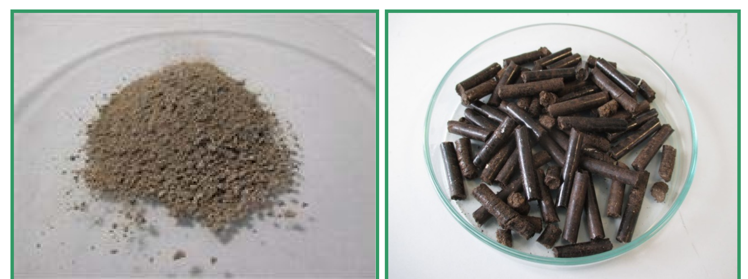
Figure 3. PhosFarm products from anaerobic digestate. Left: Precipitated phosphate salts. Right: Pellets from organic solid fraction
