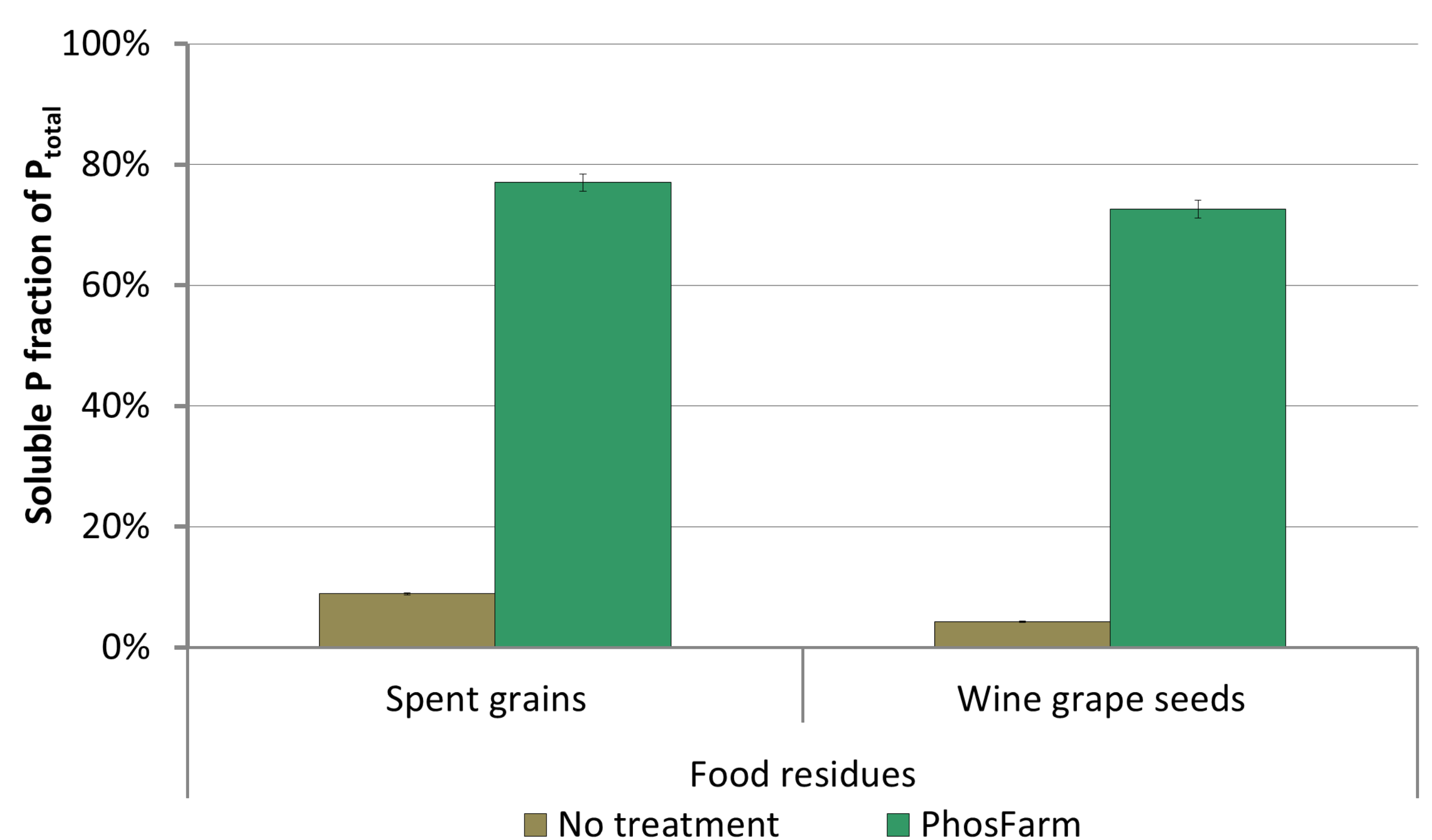
Figure 2. Increase in the soluble P concentration in food residue samples by enzymatic treatment
